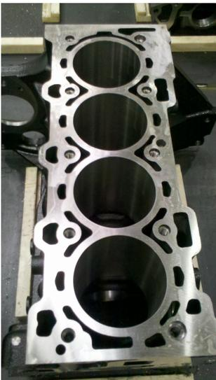
Roughing milling of a Engine Block Made of GG300
